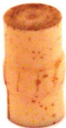
Fig. 6. Character of fatigue failure of test piece perform of Epidian 57 curing Z1 during one hour in the temperature 60°C, put under load the cycle 0.2-5 kN (about the maximum value equal 0.5 short-term compression strength)
